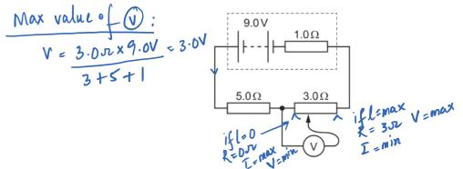
The sliding contact of the potentiometer is moved over its full range of movement.
