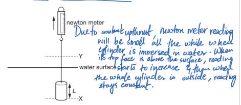
The cylinder, of height L, is slowly raised vertically by lifting the newton meter.
