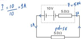
Which change occurs when the  $5.0\Omega$  load resistor is replaced with a  $50\Omega$  load resistor?
