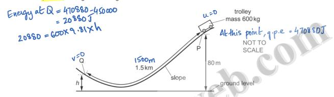
The total distance PQ moved by the trolley along the slope is 1.5 km. A constant resistive force of 300 N opposes the motion of the trolley on the slope. Work done against friction = 300 XI 500 = 450,000 J
