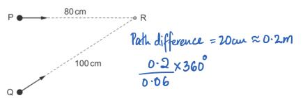
Both waves have a wavelength of 6.0 cm. The waves are in phase at point R.
