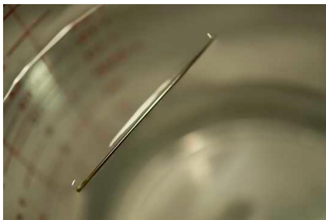
Figure 2.16 A needle's weight pulls the surface downward. At the same time, the surface tension pulls it up, suspending it on the water's surface preventing it from sinking. Notice the indentation in the water around the needle. (credit: Cory Zanker)
