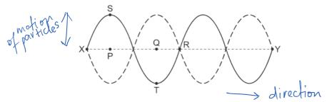
The solid curve shows the string at a position of maximum displacement. The dashed curve shows the other position of maximum displacement. The straight central dashed line shows the mean position of the string. Point S on the string is directly above point P. Point T on the string is directly below Q.
