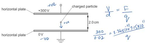
The acceleration of the particle is  $7.15 \times 10^{11} \, \text{ms}^{-2}$  downwards. The particle has a mass of  $3.34 \times 10^{-27} \, \text{kg.}$  negligible force due to weight so the only significant. What is the charge on the particle? Force could be electric force i.e downwards  $A + 1.6 \times 10^{-19} \, \text{C}$  which means the particle is tyely charged
