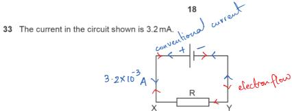
What are the direction of flow and the rate of flow of electrons through the resistor R?
