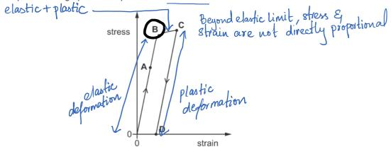
21 A tensile force is applied to an unstretched rubber band, causing it to stretch. The tensile force is then removed.
