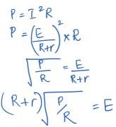
What is the maximum value of *E* if the resistor does not overheat?
