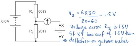
The circuit is to be used to test whether the electromotive force (e.m.f.) of a particular cell is 1.5 V. The cell is connected between terminals X and Y in parallel with R2 and in series with a galvanometer.
