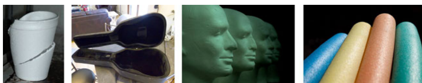
Figure 4.104: A collection of products made from polystyrene: a cup, a guitar case, polystyrene carvings, and floating pool noodles.
