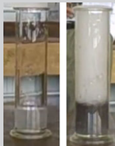
Figure 7.3: \text{H}_2\text{O}_2 before the addition of \text{MnO}_2 (left) and after the addition of \text{MnO}_2 (right).
